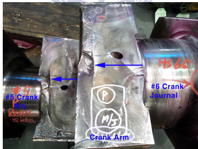
Figure 2.9 Fracture surface of the failed crank arm
