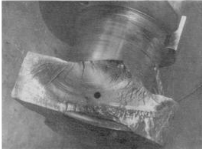
Figure 2.5 Typical bending and torsional fatigue fractures of crankshaft
