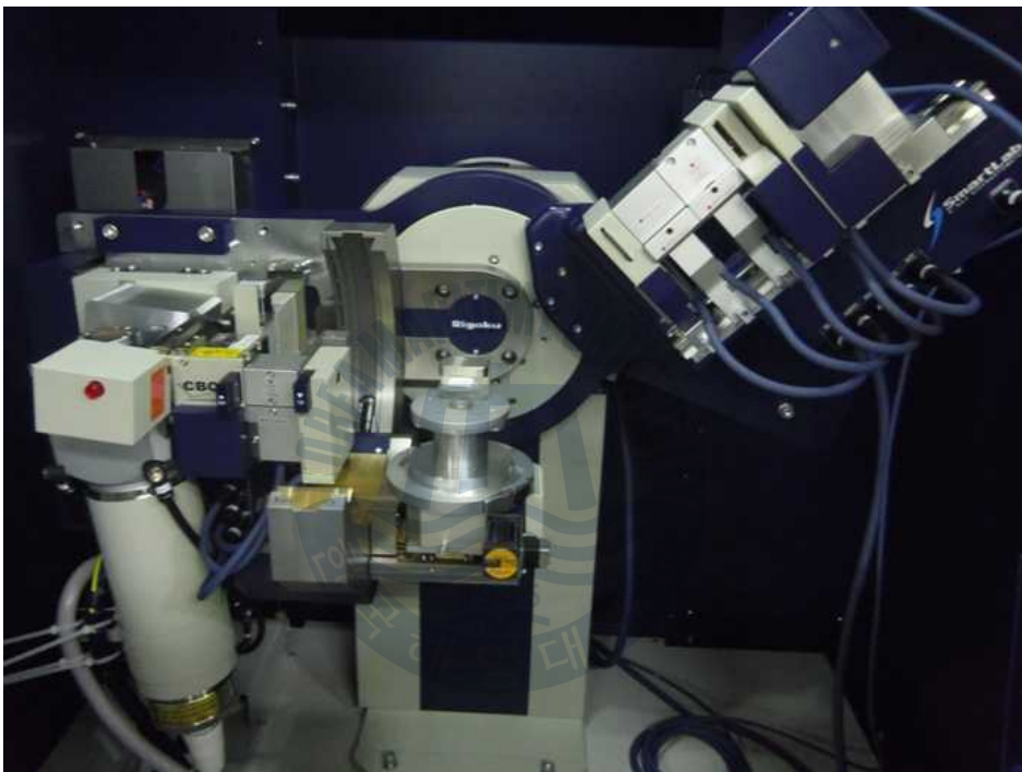
Fig. 2.2 Smartlab. high resolution powder X-ray diffraction
