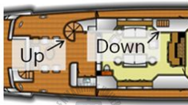
Fig. 40 External stairs: independent style
