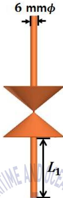
Fig. 2.3 Antenna structure with variation of  $L_1$ .
