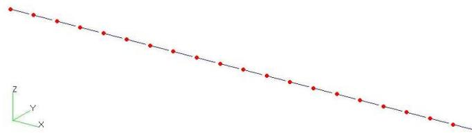
(a) Finite element mesh model (1-D)
