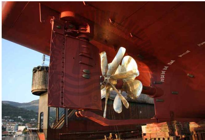
Fig. 3.26 Vane wheel installed on propeller cap<sup>[18]</sup>
