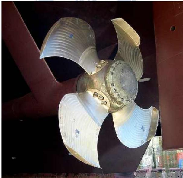
Fig. 3.5 CLT (Contracted and Loaded Tip)
