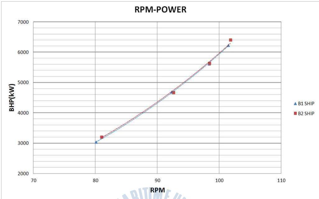
Fig. 5.11 RPM-Power for B1 ship and B2 ship
