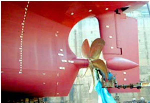
Fig. 3.22 Mitsui Integrated Propeller Boss of MES
