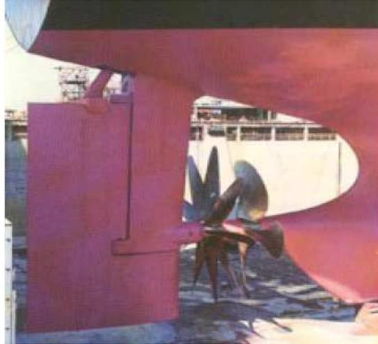
Fig. 3.27 Vane wheel installed on rudder horn
