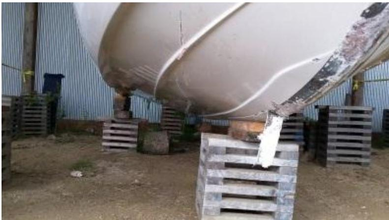
Fig.2.9 Impact Damage
