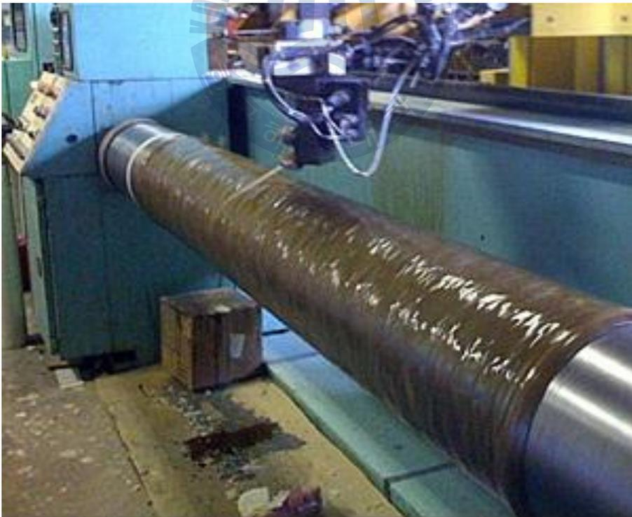
Fig.2.3 Filament Winding Process
