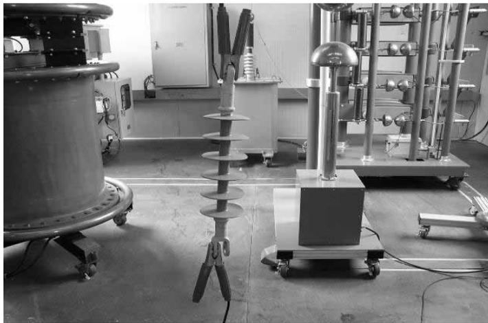
**Fig. 63** Radio influence voltage test (After injection).
