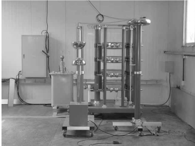
Fig. 66 Critical impulse flashover test machine.
