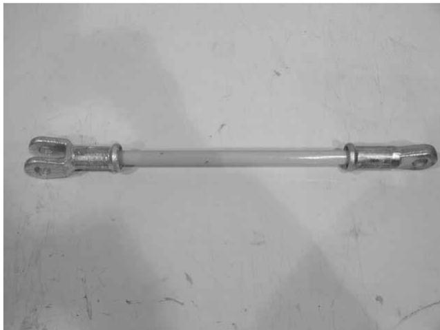
Fig. 60 Zero-defect FRP insulating rod.
