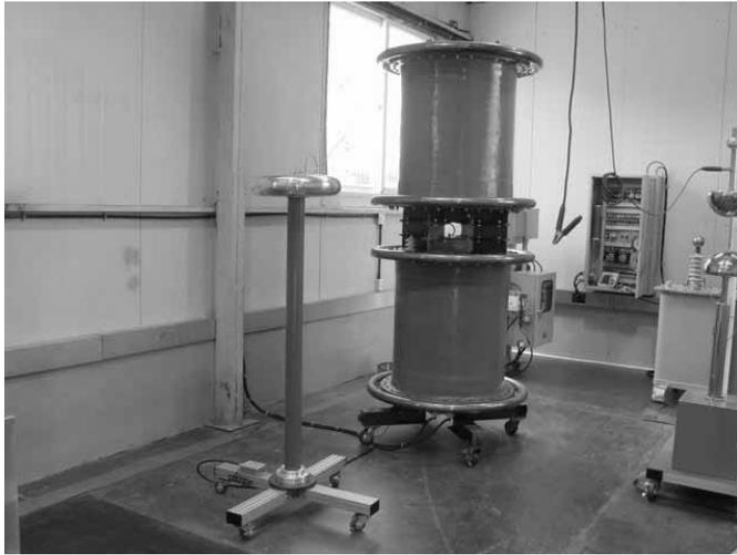
Fig. 61 Radio influence voltage test machine.
