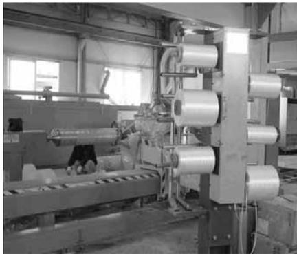
Fig. 7 4 axis Filament winding machine.
