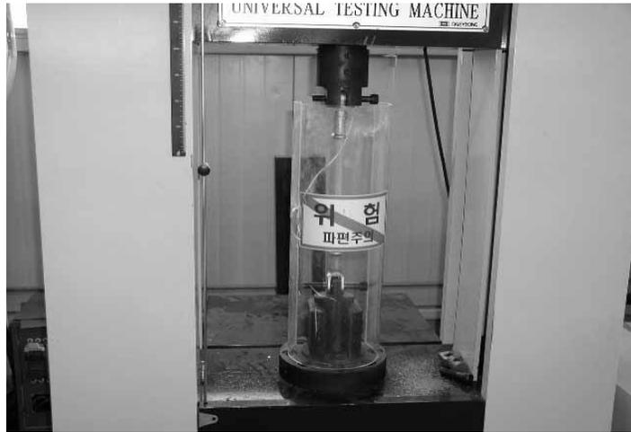
Fig. 28 Tensile fracture load test
