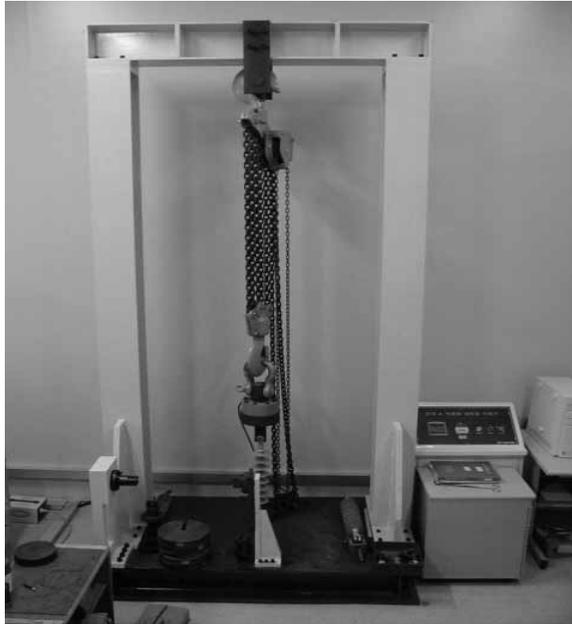
Fig. 45 Mechanical load-time test machine.
