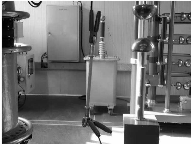
Fig. 67 Critical impulse flashover test.
