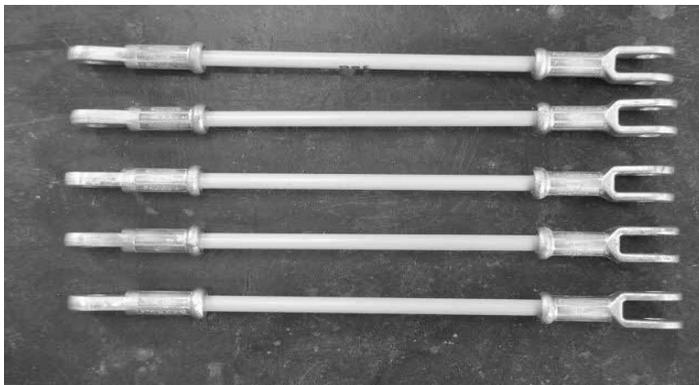
Fig. 27 Tensile fracture load test specimen.
