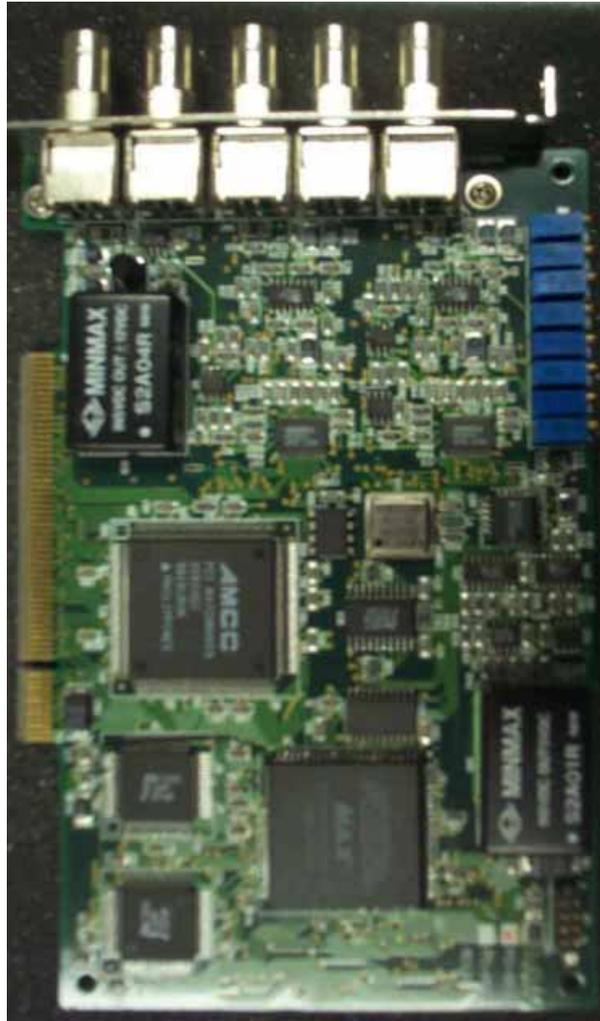
Fig.4.11 Data Acquisition Board
