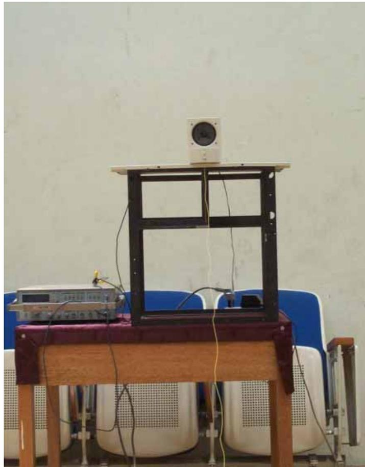
Fig.4.6 Sound Signal Transmitting Part Using Audio Generator
