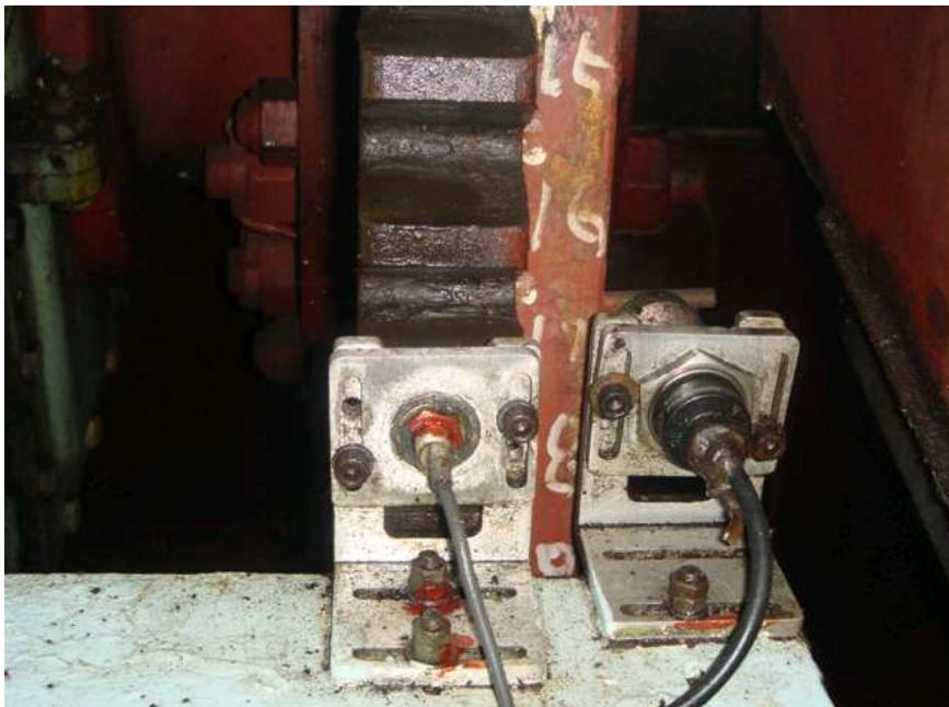
Fig. 3.2 Tooth & TDC(trigger) sensor on the flywheel
