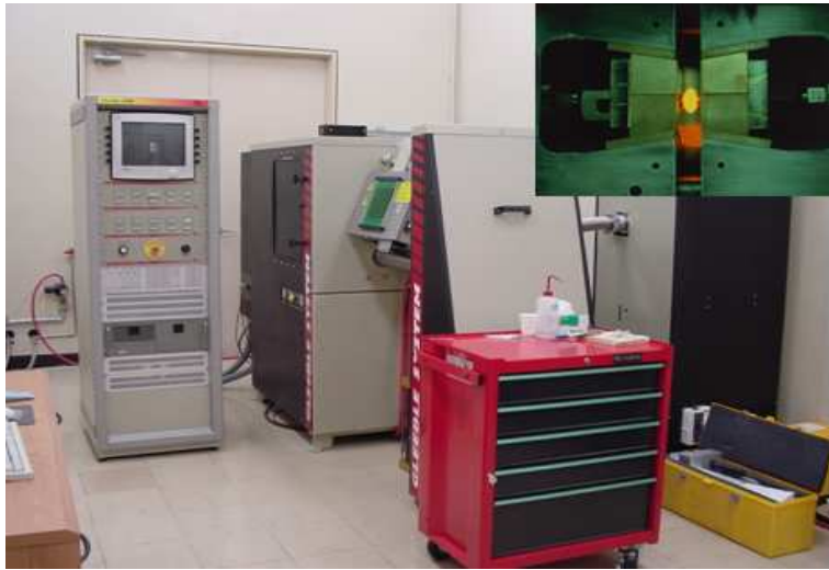
Figure 9. Appearance of GLEEBLE SYSTEM and fixtures with specimen installed.
