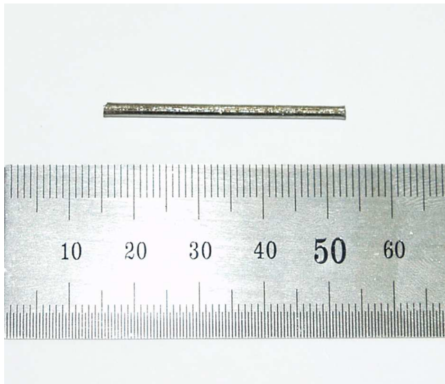
Figure 3. Image of (a) \text{Fe}_{43.8}\text{Mn}_{10.7}\text{Mo}_{12.7}\text{Cr}_{15.6}\text{B}_{5.6}\text{Y}_{1.5}\text{Co}_{4.9} alloy (as cast) and (b) \text{Fe}_{56}\text{Co}_{5.6}\text{Si}_{2.4}\text{Zr}_{6.5}\text{B}_{13.5} alloy (as cast).
