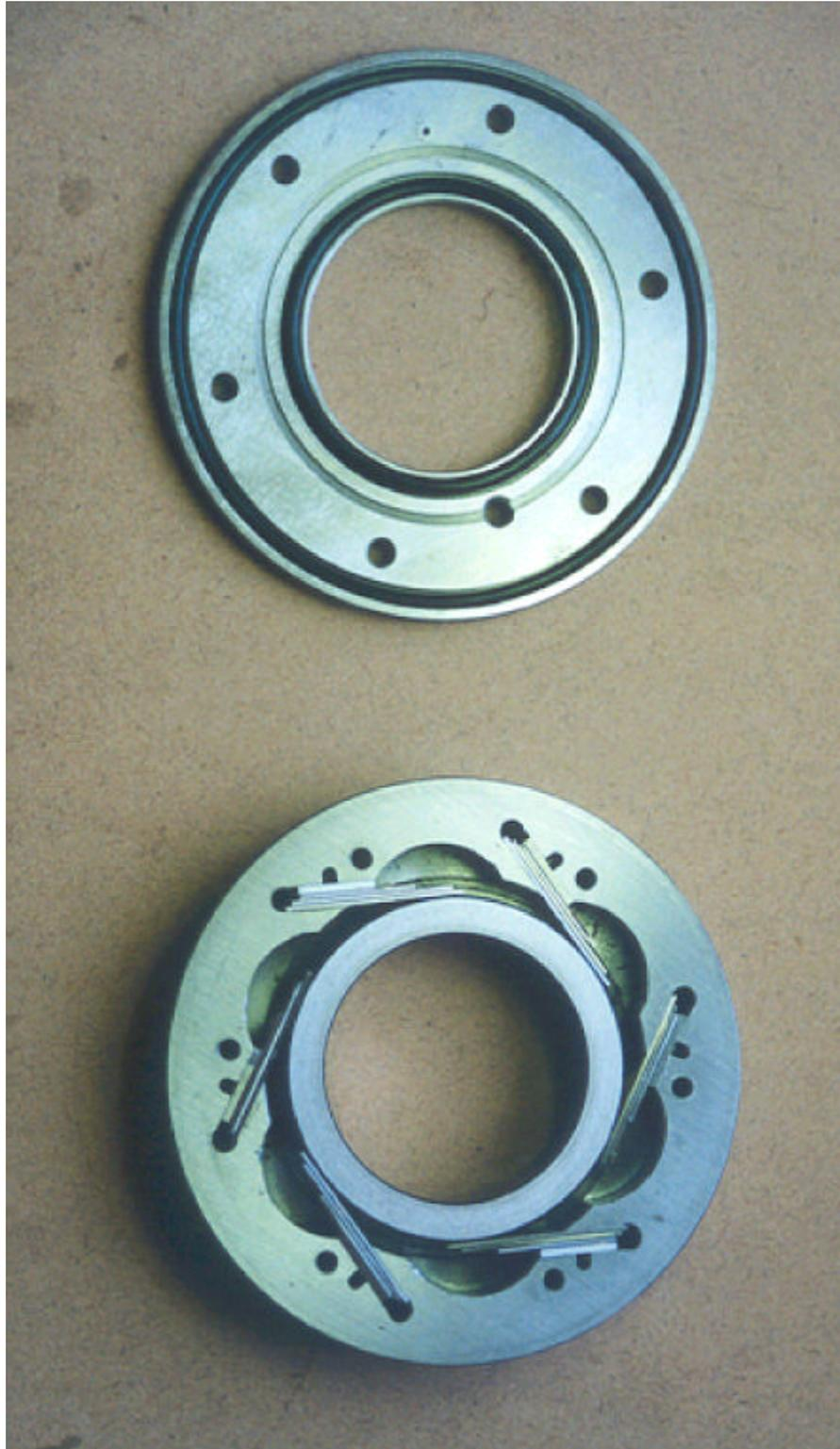
Fig.4.2 Photography of Leaf Spring Damper (Type C)
