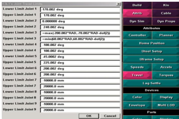
Fig. 5.3 Joint Travel Limits
