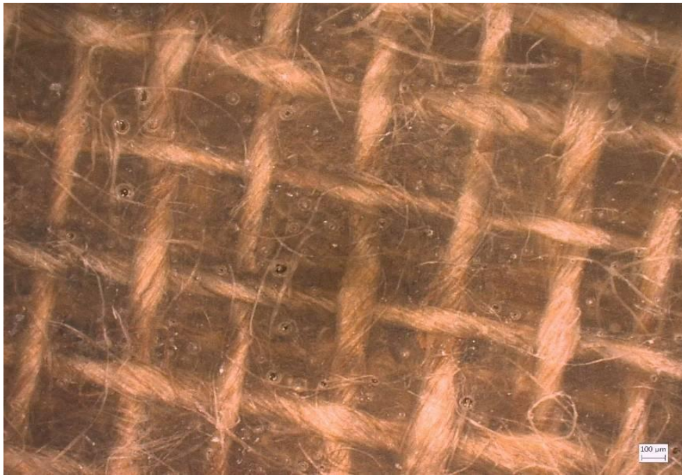
(a) Surface made by hand lay-up
