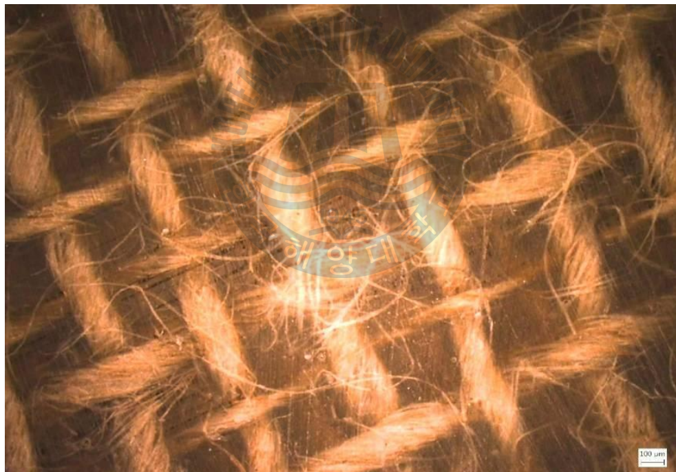
(a) Surface made by VARTM
