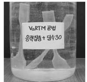
Fig. 4-19 VaRTM (notched specimen) Temp.: 22°C
