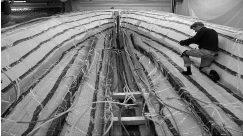
Fig. 2-2 Ship building process by VaRTM
