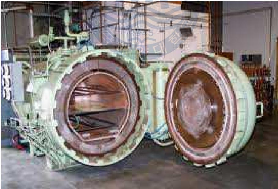
Fig. 4 Picture of autoclave process
