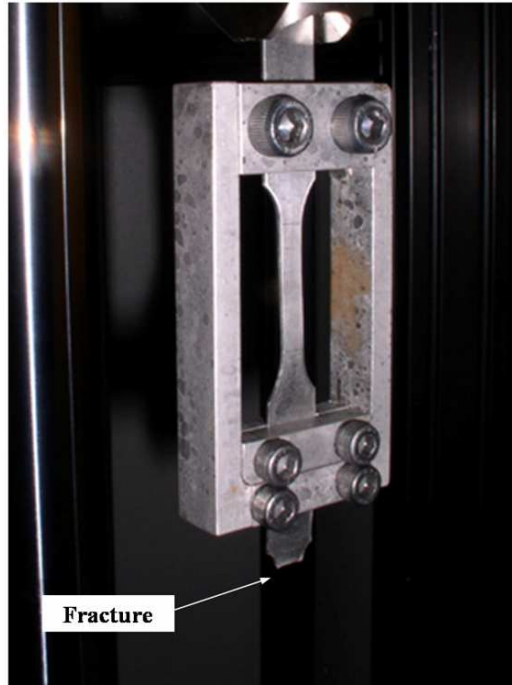
Fig. 14 Fractured specimen with stopper mounted in the testing machine.
