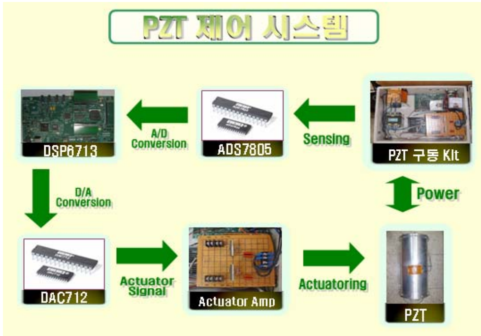
Fig 2.1 Control system using DSP processor
