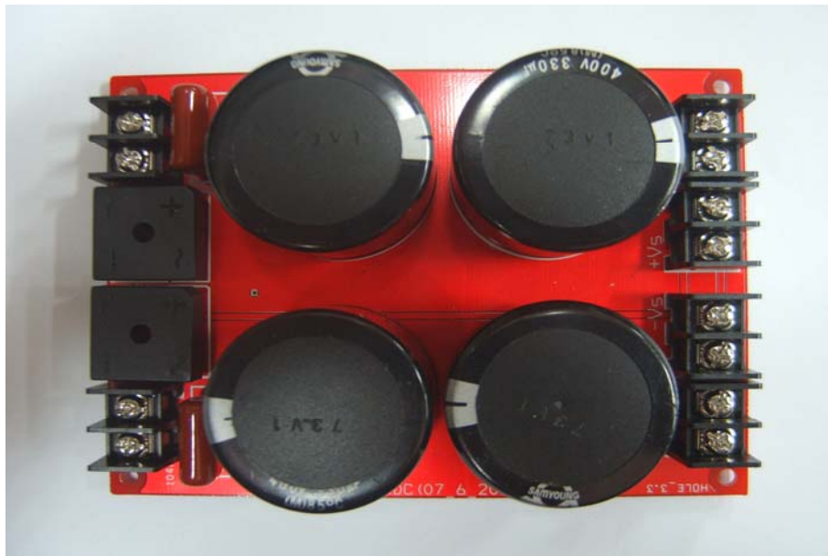
Fig 5.4 The PCB of the Bridge Circuit
