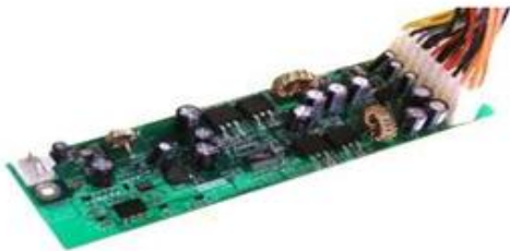
Fig. 10 Power supply board
