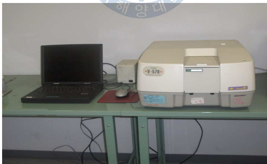
Fig. 14 The figure of UV-VIS-NIR spectrometer (V-570, Jasco)
