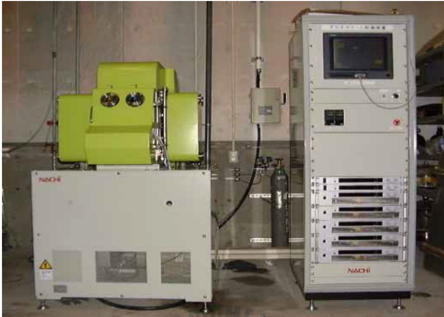
Fig. 11 The inclination opposite target type DC magnetron sputtering equipment
