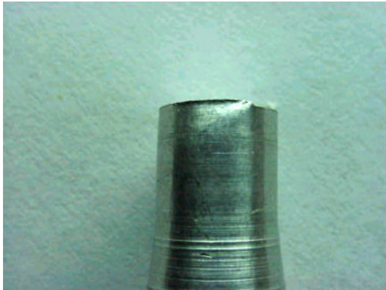
Photo 9 Shape of fracture at 748 803K
