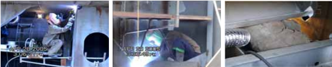
(a) Overhead welding posture (b) Flat welding posture I (c) Flat welding posture II
