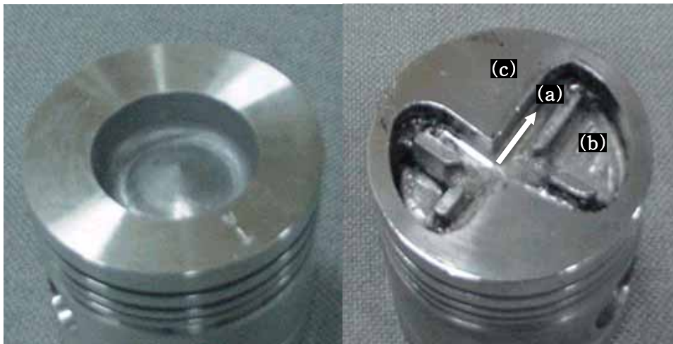
a) Conventional high swirl piston b) 2-stage combustion piston
