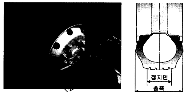
Fig. 3 Earthing shape of tire, total width and real earthing width of tire
