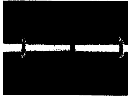
Fig.2 Modulation Type Noise after BPF(X:2ms, Y:0.2V)
