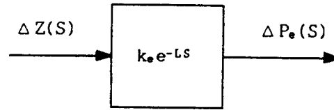
Fig. 2.4 Block Diagram of an Engine
