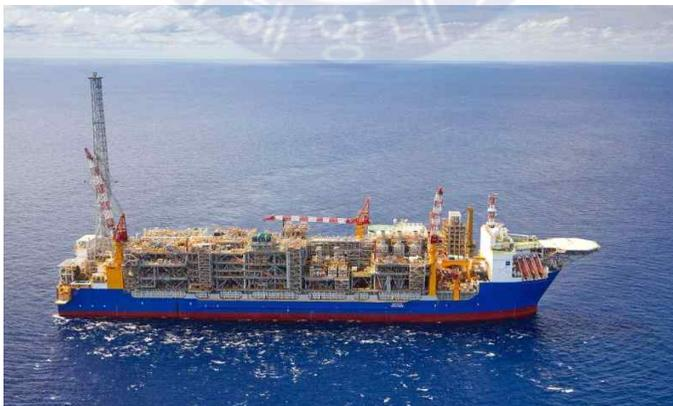
(b) FPSO (Floating, Production, Storage and Offloading)
