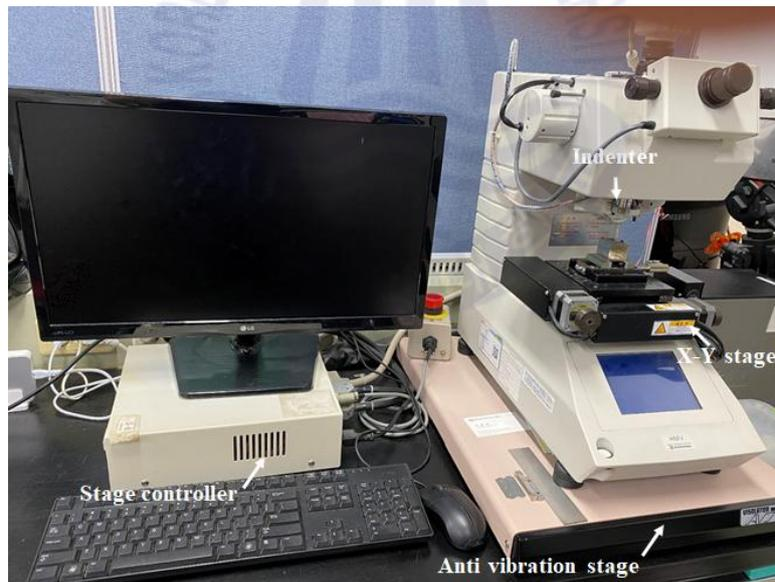
Fig. 3.7 Photograph of hardness tester
