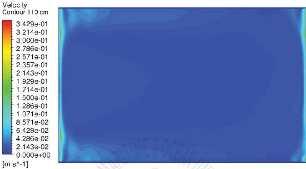
Fig. 4.19 Off-mode air velocity contour on Z = 1.1 m horizontal plane
