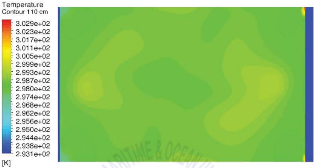
Fig. 4.17 On-mode air temperature contour on  $Z = 1.1$  m horizontal plane
