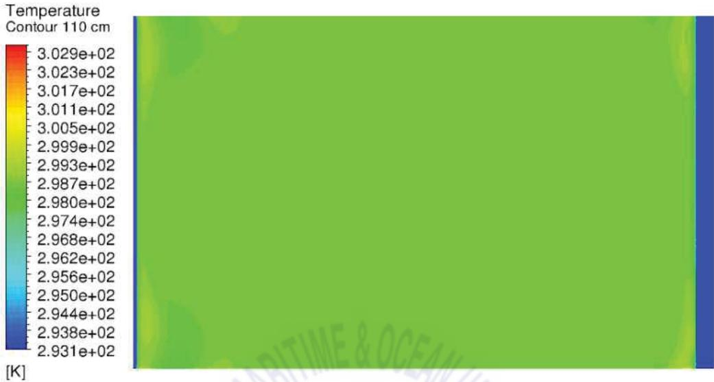
Fig. 4.21 Off-mode air temperature contour on  $Z = 1.1$  m horizontal plane
