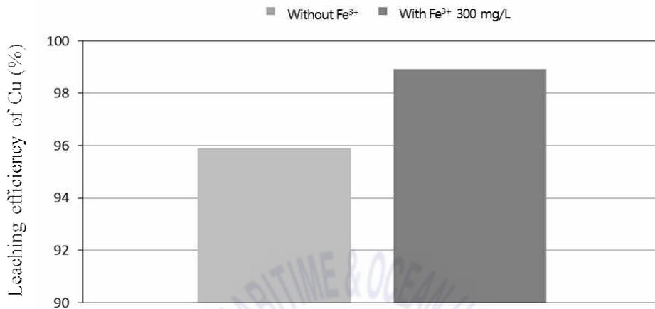
**Fig. 16** Leaching efficiency of Cu with variation of Fe<sup>3+</sup> concentration
