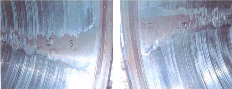
Fig. 2.1 An example of the damage of after stern tube bearing
