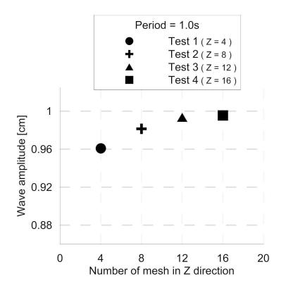
Fig.4 Mesh sensitivity test (Choi & Lee, 2017)
