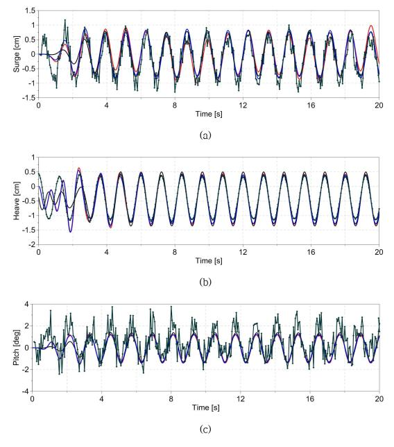
Fig.11 Time history of (a) Surge, (b) Heave, and (c) Pitch motion response (Period = 1.2s, Amplitude = 0.02m)
