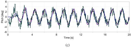
Fig.17 Time history of (a) Surge, (b) Heave, and (c) Pitch motion response (Period = 1.6s, Amplitude = 0.06m)
