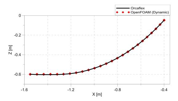
Fig.9 Profile of mooring line after static calculation
