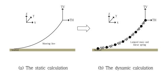
Fig.6 The two calculation stages
