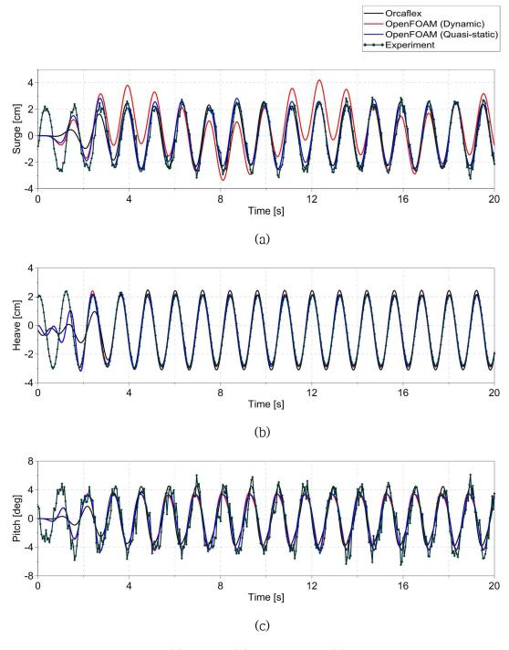
Fig.15 Time history of (a) Surge, (b) Heave, and (c) Pitch motion response (Period = 1.2s, Amplitude = 0.06m)
