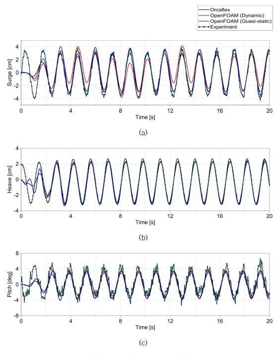
Fig.16 Time history of (a) Surge, (b) Heave, and (c) Pitch motion response (Period = 1.4s, Amplitude = 0.06m)
