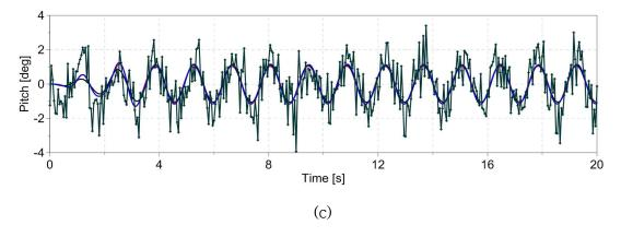
Fig.12 Time history of (a) Surge, (b) Heave, and (c) Pitch motion response (Period = 1.4s, Amplitude = 0.02m)
