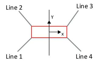
Fig.7 Mooring line lay-out
