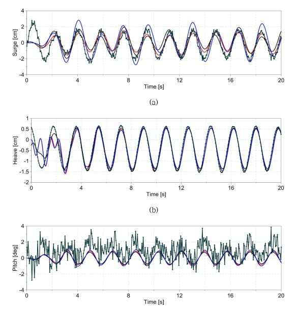
Fig.14 Time history of (a) Surge, (b) Heave, and (c) Pitch motion response (Period = 1.8s, Amplitude = 0.02m)
