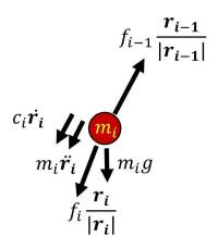
Fig.8 Force diagram acting on a lumped mass
