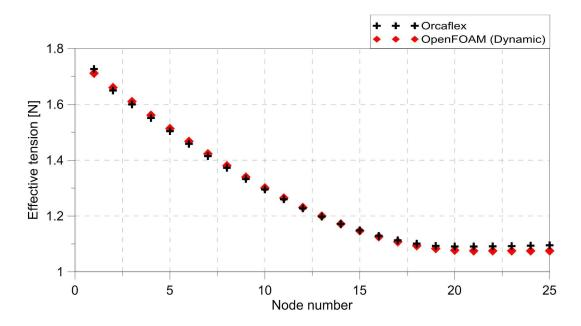
Fig.10 The tension acting on the lumped mass of Line 1  $\,$
