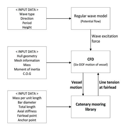
Fig.1 Coupled analysis diagram
