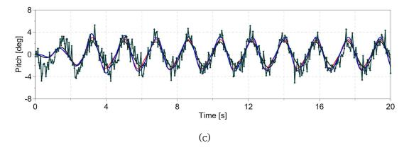
Fig.18 Time history of (a) Surge, (b) Heave, and (c) Pitch motion response (Period = 1.8s, Amplitude = 0.06m)
