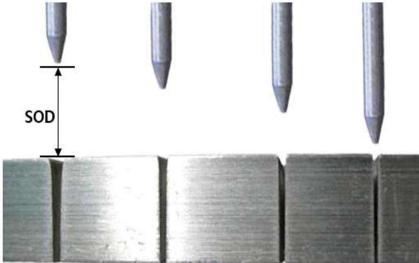
Fig. 10 Quality level in accordance with SOD Change
