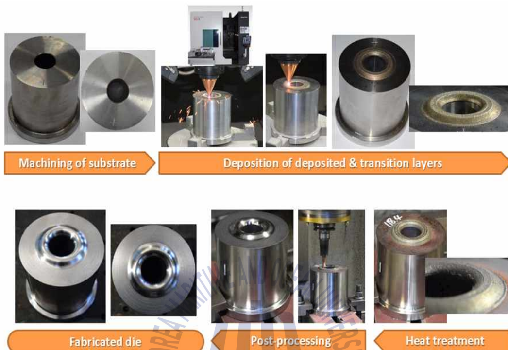
Fig. 5-1 Deposition process of hot forging die
