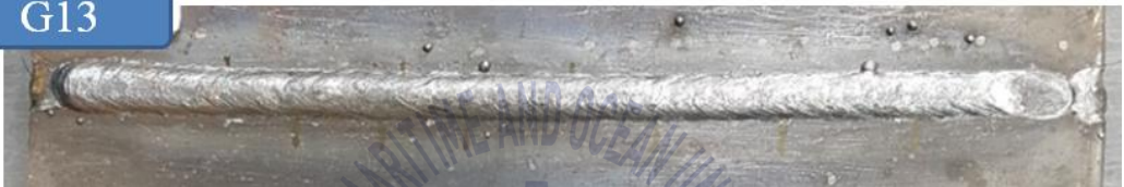
Fig.35 Weld bead of specimen having 1.6mm gap and coated with grease - 3
