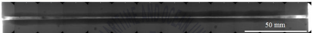
Fig.64 RT result of weld bead having 1.6mm gap and filled with slag pieces - 2
