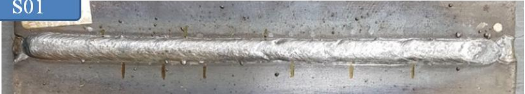
Fig.38 Weld bead of specimen having no gap and filled with slag pieces - 1
