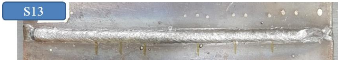
Fig.42 Weld bead of specimen having 1.6mm gap and filled with slag pieces - 3
