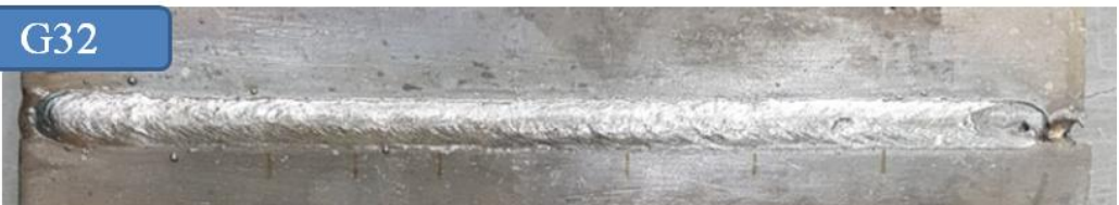
Fig.37 Weld bead of specimen having 3mm gap and coated with grease - 1
