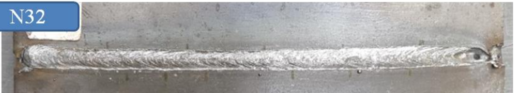
Fig.30 Weld bead of specimen having 3mm gap and no defects - 2
