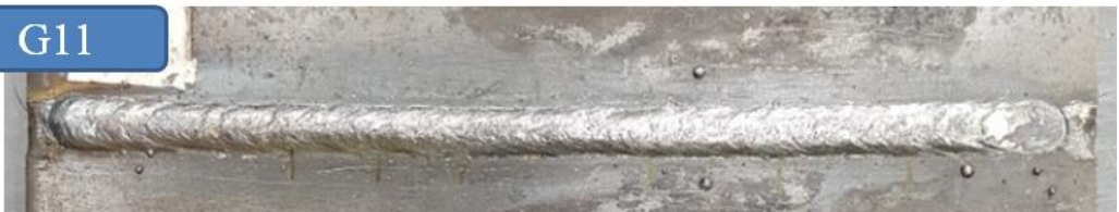
Fig.33 Weld bead of specimen having 1.6mm gap and coated with grease - 1
