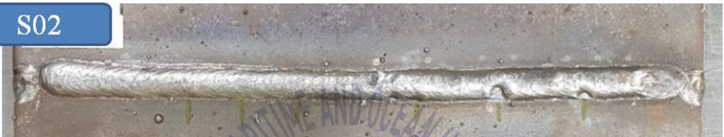
Fig.39 Weld bead of specimen having no gap and filled with slag pieces - 2
