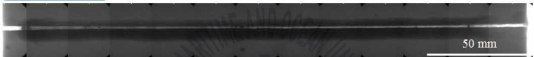
Fig.57 RT result of weld bead having 1.6mm gap and coated with grease - 2
