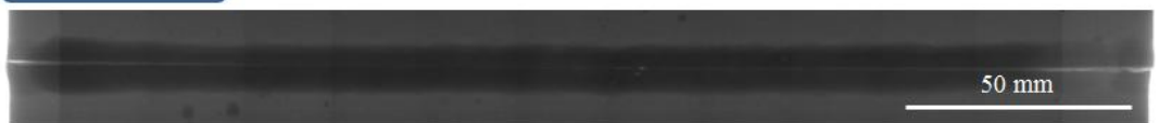
Fig.55 RT result of weld bead having no gap and coated with grease - 2
