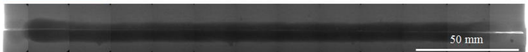
Fig.54 RT result of weld bead having no gap and coated with grease - 1
