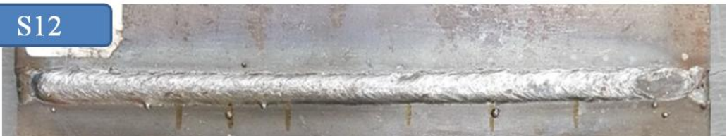
Fig.41 Weld bead of specimen having 1.6mm gap and filled with slag pieces - 2
