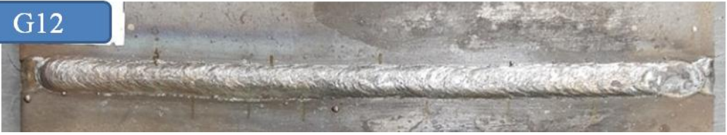
Fig.34 Weld bead of specimen having 1.6mm gap and coated with grease - 2
