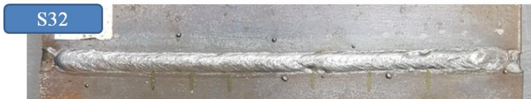
Fig.45 Weld bead of specimen having 3mm gap and filled with slag pieces - 2
