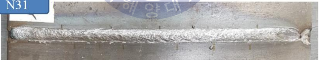
Fig.29 Weld bead of specimen having 3mm gap and no defects - 1
