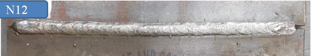
Fig.28 Weld bead of specimen having 1.6mm gap and no defects - 2
