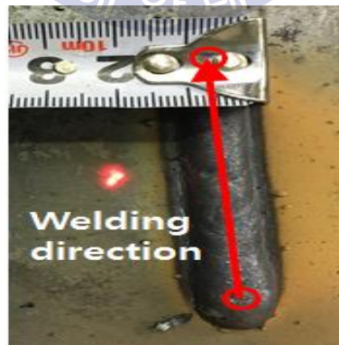
Fig.5 1st measuring of HAZ(15mm far from center of the bead)
