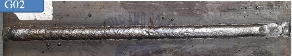
Fig.32 Weld bead of specimen having 0mm gap and coated with grease - 2
