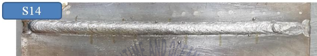
Fig.43 Weld bead of specimen having 1.6mm gap and filled with slag pieces - 4
