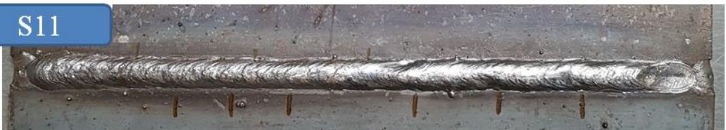
Fig.40 Weld bead of specimen having 1.6mm gap and filled with slag pieces - 1
