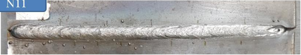
Fig.27 Weld bead of specimen having 1.6mm gap and no defects - 1
