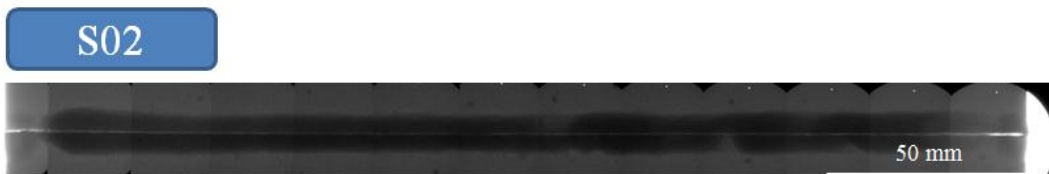
Fig.62 RT result of weld bead having no gap and filled with slag pieces - 2
