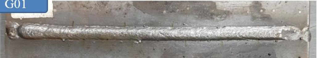
Fig.31 Weld bead of specimen having 0mm gap and coated with grease - 1
