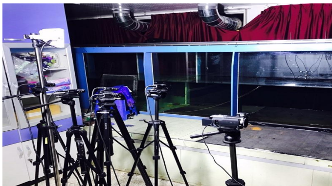
Fig. 11 3D Displacement meter
