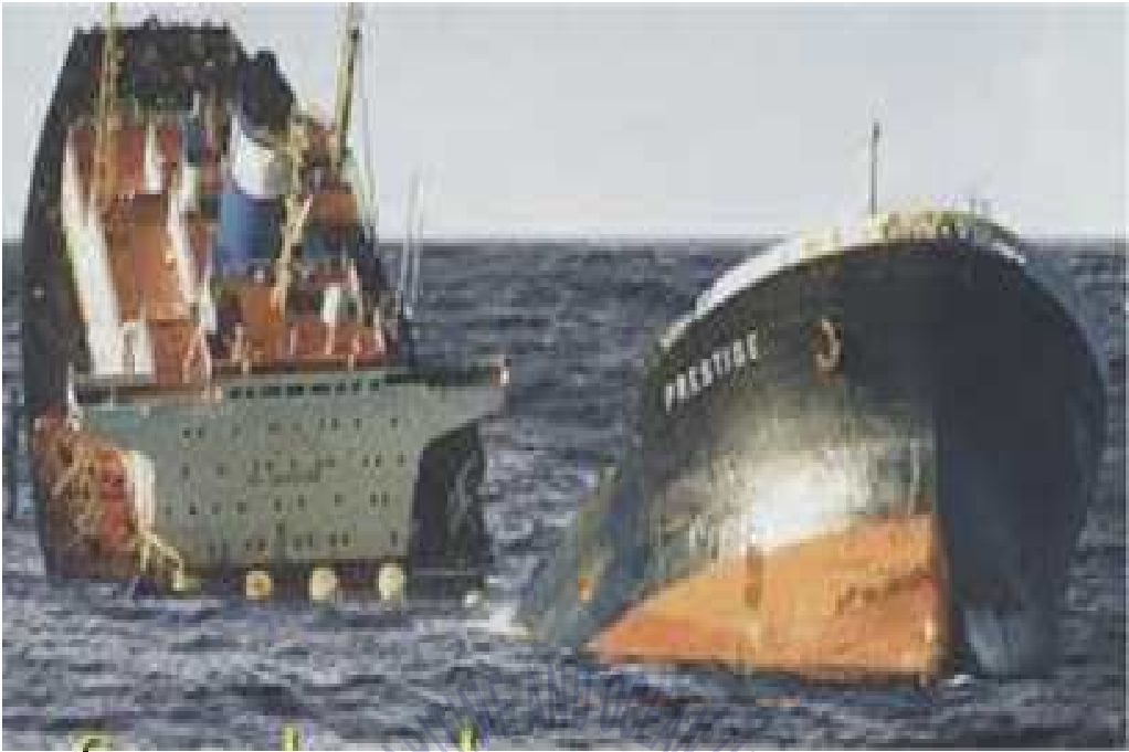
Fig. 14 MT“Prestige”broken in two
