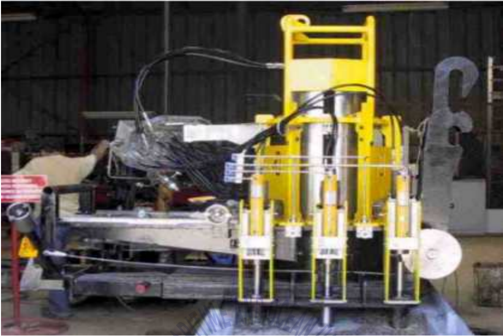
Fig. 16 Special designed Hot tapping machine for “Prestige”project
