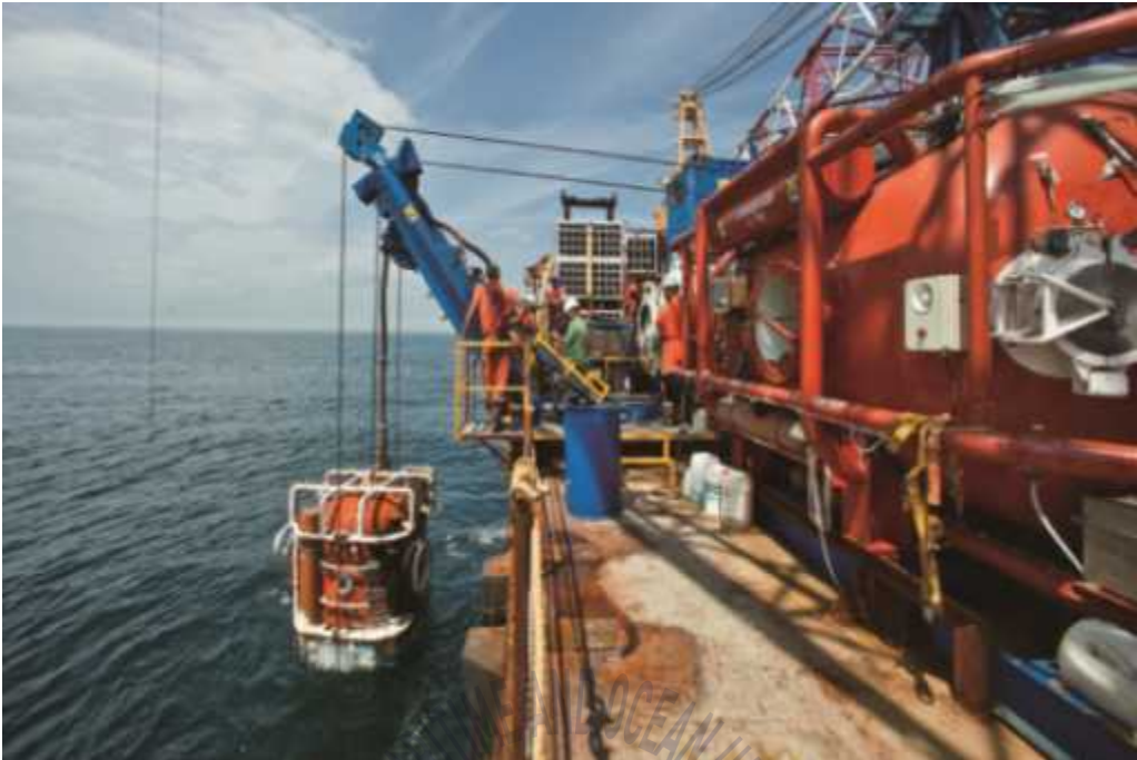
Fig. 9 Launching diving bell for saturation diving
