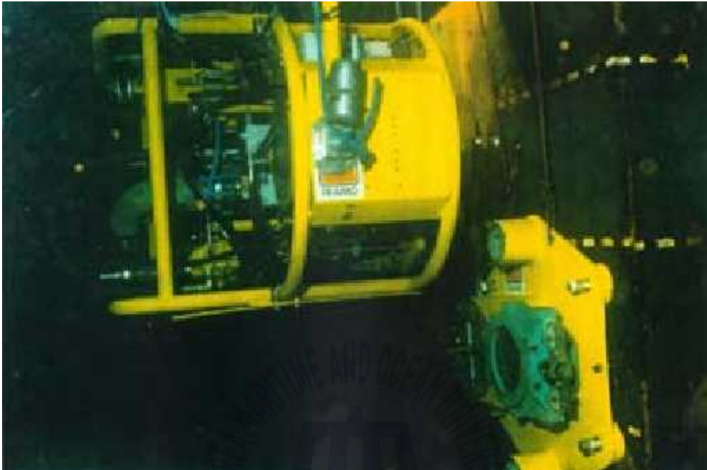
Fig. 7 Releasing ROLS after attached Base Plate
