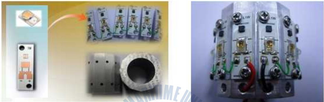
Fig. 2 Prototype of High Brightness LED Module
