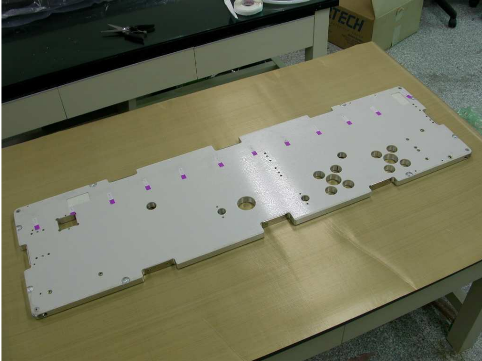
Fig. 31 Completed transportation rack by press process
