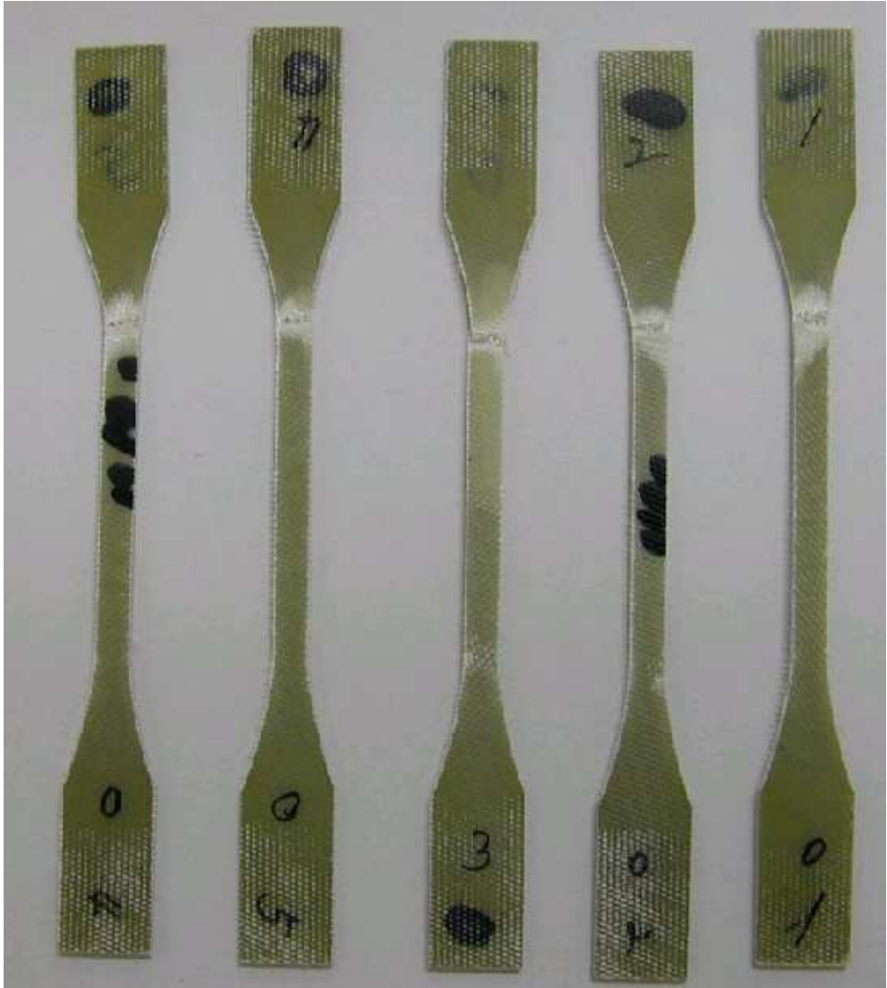
Fig. 38 Fractured specimens of tensile test
