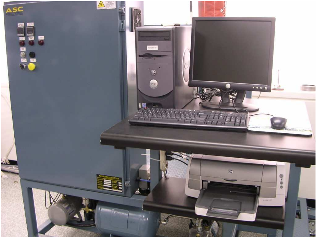
Fig. 23 Control system for autoclave
