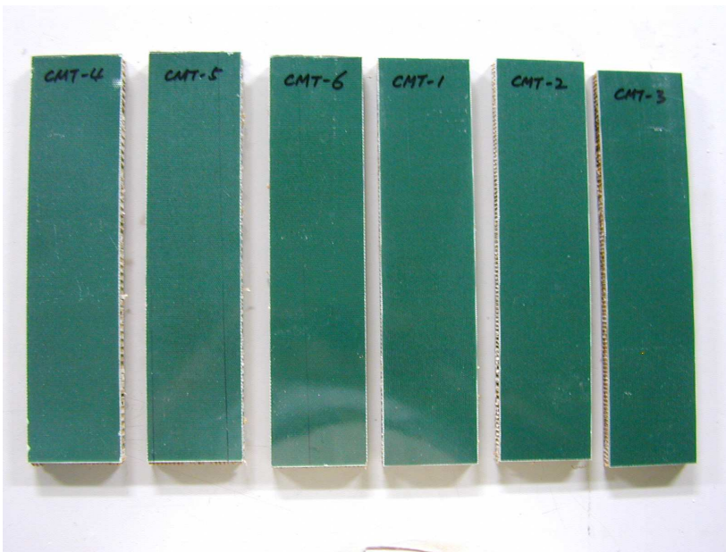
Fig. 44 Specimens for long beam flexural test
