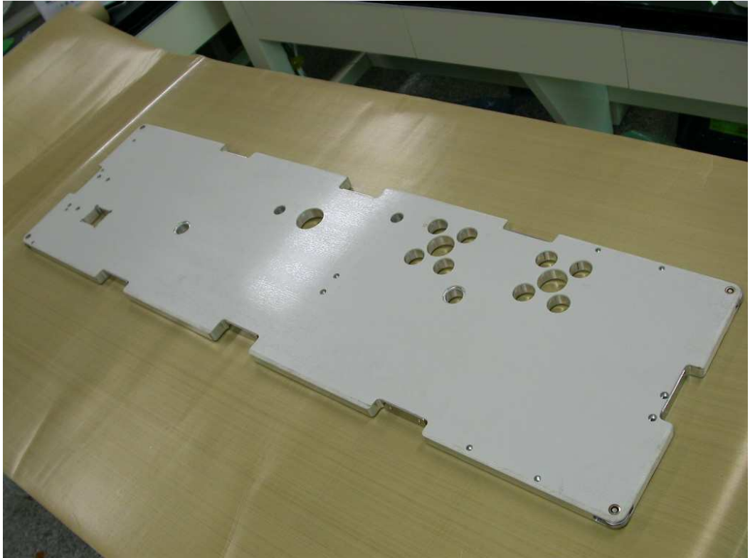
Fig. 27 Completed transportation rack by autoclave process
