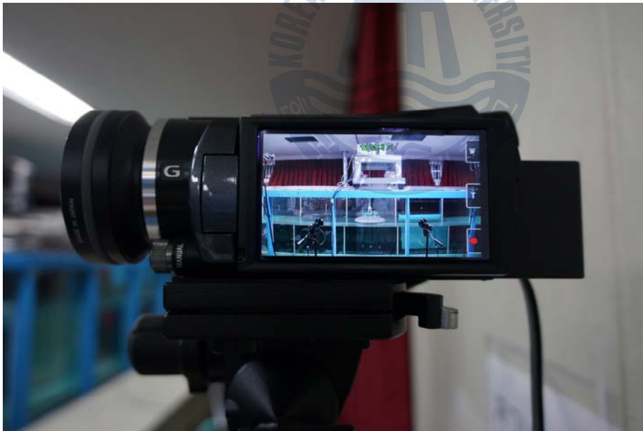
Fig. 3.17 Video camera set up to record motion of buoy under test
