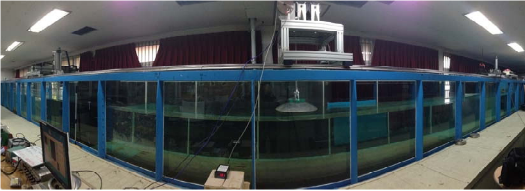
Fig. 3.2 Set up of 1:20 scale WEC model on the basin
