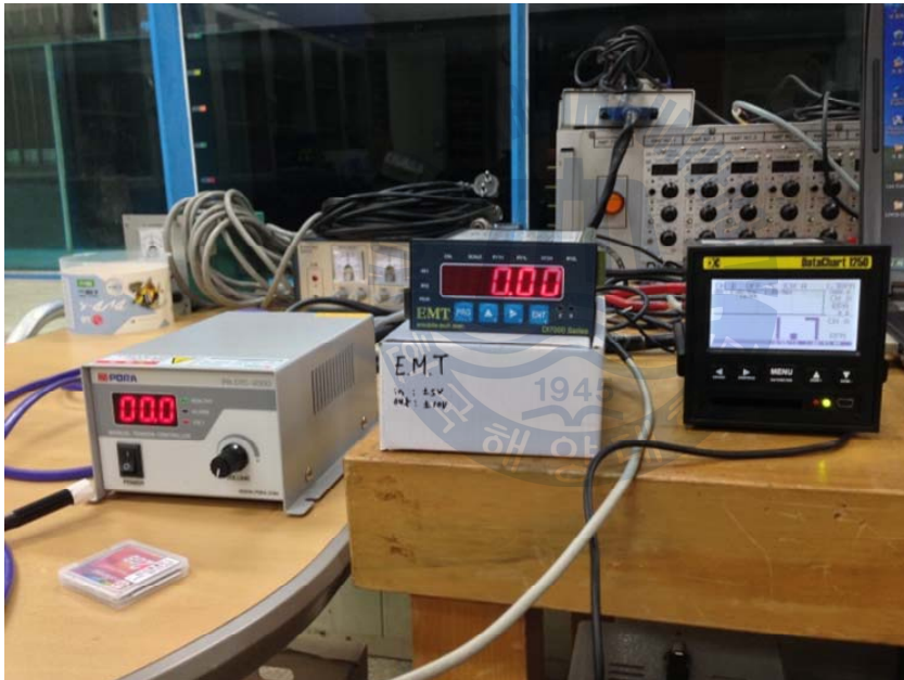
Fig. 3.10 Brake controller to increase load to rotary axis(left). Torque indicator(center) and RPM indicator(right) to monitor measuring torque and RPM real time under test
