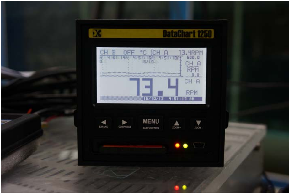
Fig. 3.18 RPM indicator set up to monitor measuring real time speed of rotary axis under test
