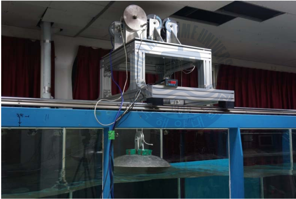
Fig. 3.3 Overview of 1:20 scale WEC model on the basin
