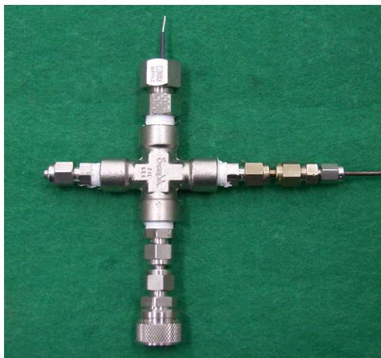
Fig. 9. External Pressure Balanced Reference Electrode assembly.
