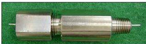
Fig. 10. Assembled specimen for LPR test (Working Electrode).
