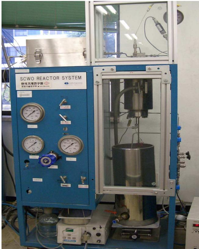
Fig. 13. SCWO reactor system for coupon test.
