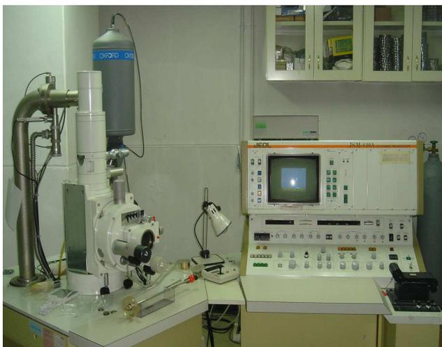
Fig. 14. Scanning electron microscope and energy dispersive X-ray spectroscope.
