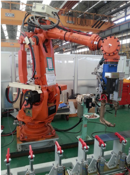
Fig. 5 Servo gun-type spot welding system. (HX200-Hi4a)
