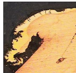
Fig. 14 Severe macro-deformation or mushrooming on a truncated cone electrode optical micrographs of electrodes tested to 1000 welds. [16]
