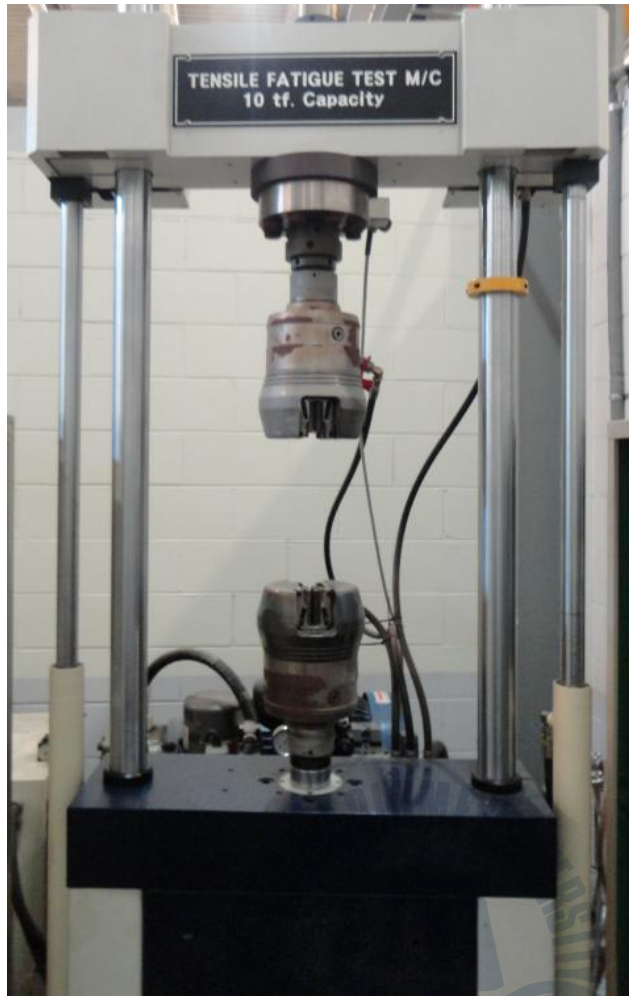
Fig. 6 Hydraulic servo fatigue test machine (KDMT-320-5).
